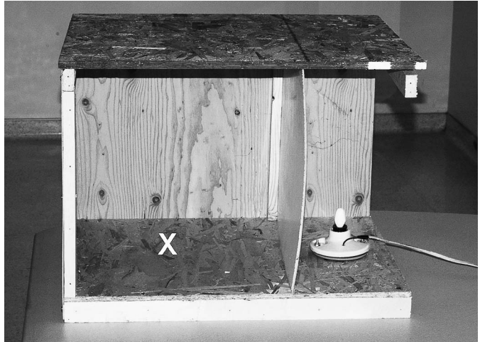
Figure 1.—View of the plywood box that housed either the 14:10 or 10:14 light cycle cohorts of spiders. The right wall of the box (facing the camera) is removed for photographic purposes. The light was placed outside of the area of the box housing the spiders and was open to the back. Spiders, in vials, were placed near the “X”.
